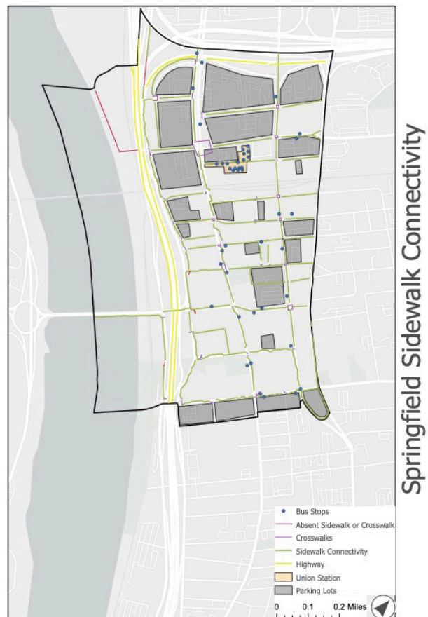
Figure 14: Field map of West Springfield study area including bus stops, sidewalks, crosswalks, and missing infrastructure.
